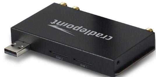
Fig. 7: Cradlepoint MC400 for the AER Series
