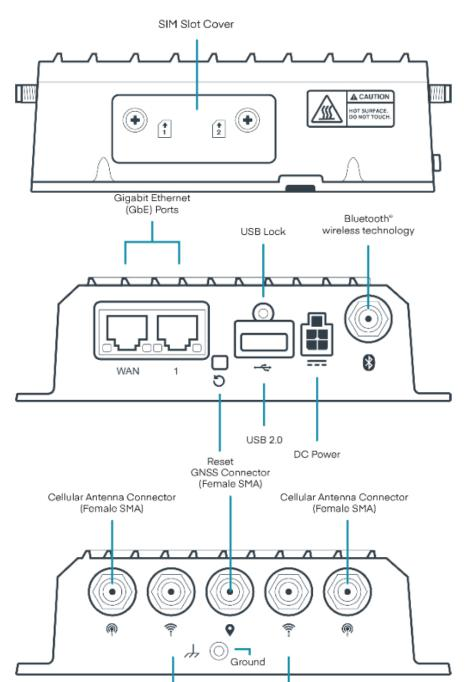
Wi-Fi Antenna Connector (Female RP-SMA)
